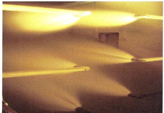
Ultimix Nozzles with Air-Cooled Spray Lance Assemblies in a non-ferrous—horizontal hot gas cooling chamber
