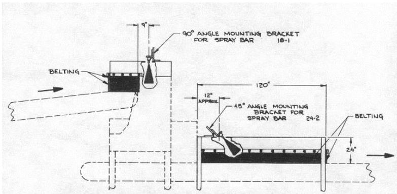
Figure 2. Typical Transfer Point Treated by Fog Nozzles
