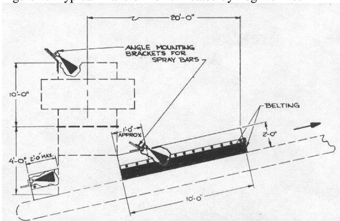
Figure 3. Typical Crusher Transfer Point Treated by Fog Nozzles
