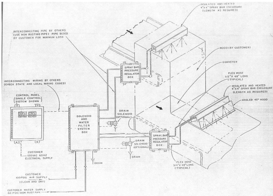
Figure 4. Typical Dust Suppression System
