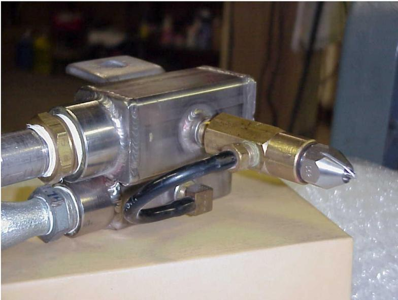
Figure 6. Typical Spray Bar Manifold with Ultimix™ Nozzle (Single Point)
