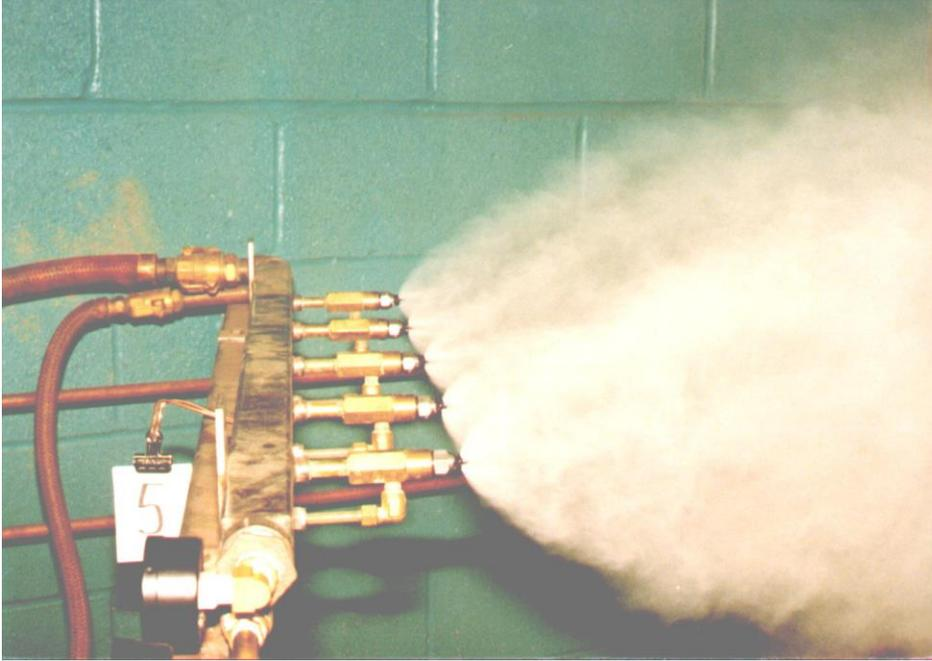
Figure 7. An array of UltraFine Fogging Nozzles.
