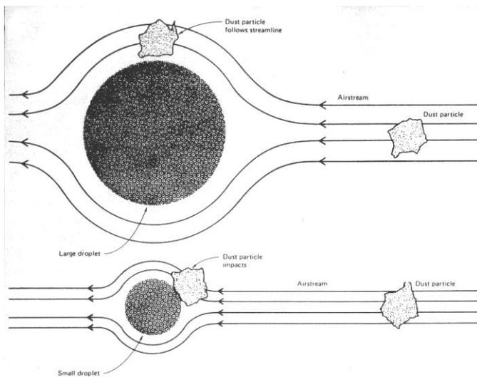
Figure 1. Theory of Agglomeration (Air Flow Around Water Droplets)
